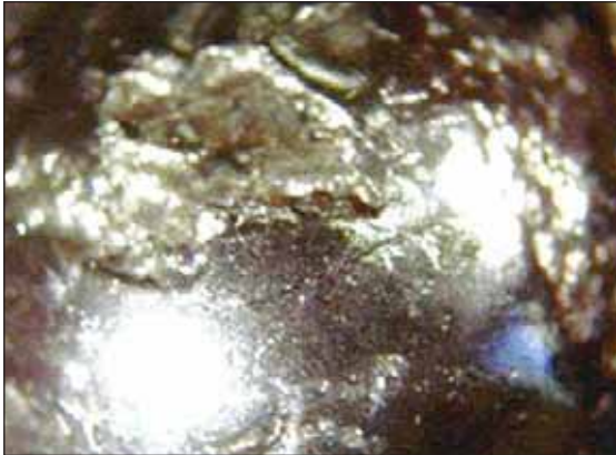
Ball With Large Crack
