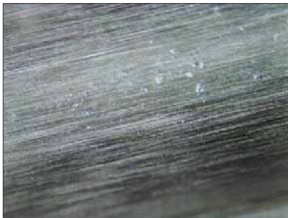
Figure 1. MICROGRAPH OF DENTS IN BALL RACEWAY OF STAND
